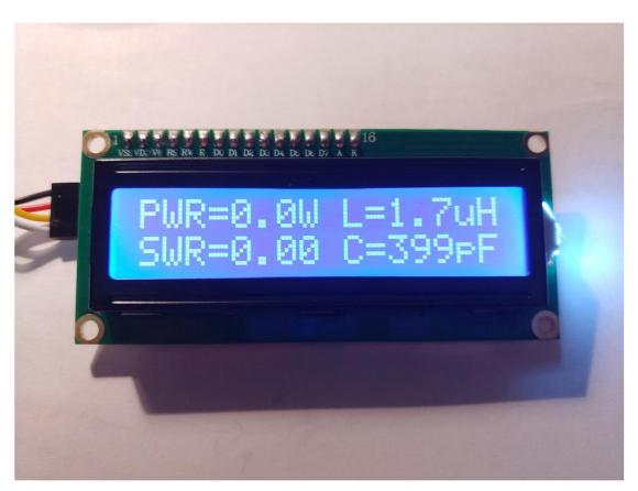
The left side of the indicator displays the power throughput and SWR. The peak detector mode is used, which allows to accurately measure the signal power of the transmitter when using various types of modulation.
